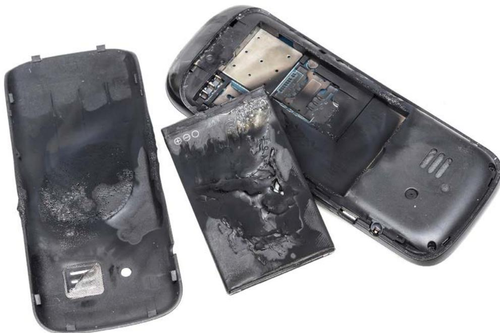
The standard requires that batteries be designed to prevent abnormal temperature rise conditions
